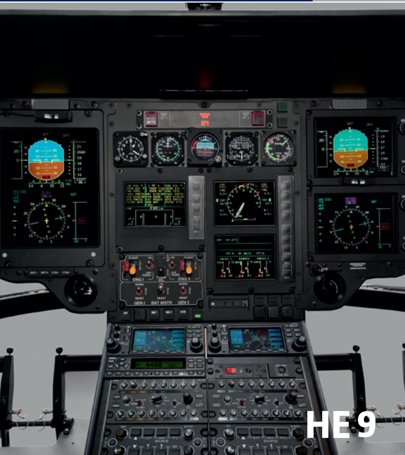
Example of H135 Flight Navigation Display (FND)
